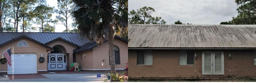
Picking a quality metal roof and using a reputable contractor to install it is important. Above right, an inferior metal roof with a subquality paint system grew fungus. The homeowners replaced it with a Drexel Metals roof in Mansard Brown (above left).
